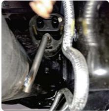
**Step 5:** Move to the front canister connection to the downpipe. Loosen the nut on the V band clamp until the clamp can be removed and now the canister can be removed from the truck. Note: Retain the factory gasket for reuse.
