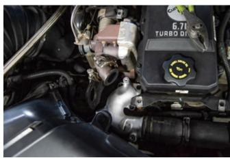
STEP 20: Install the coolant bypass hose to the coolant bypass elbow.
