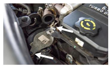
STEP 16: Using a pair of channel locks, loosen the clamp that retains the coolant hose to the coolant elbow. Slide it down the coolant hose to allow for removal of the hose from elbow.
