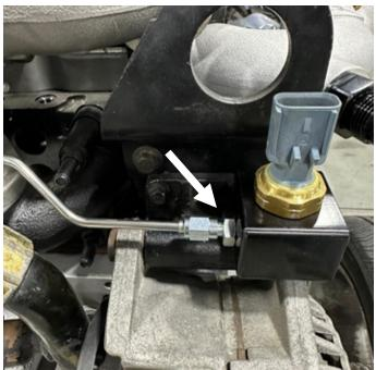
STEP 27: Install and connect the back pressure sensor line at both the exhaust manifold and at the sensor block. Reconnect the exhaust back pressure sensor to the chassis harness.
