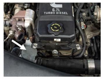
STEP 22: Use the double hose clamps provided in the kit to secure the coolant bypass hose to the coolant riser line.
