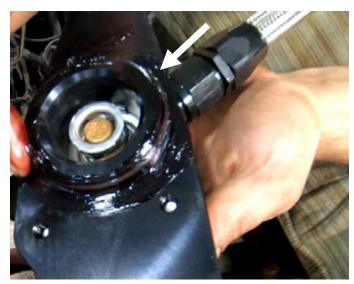
STEP 7: Slide the thermostat housing between the firewall and the back of the engine block. Align the thermostat housing with the original freeze plug hole location and press the housing against the engine to seat the housing. The coolant bypass hose should be oriented towards the passenger side of the vehicle.
