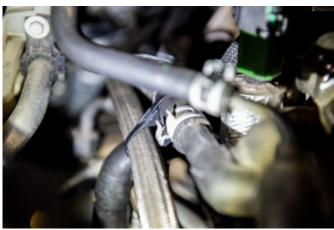
STEP 23: Reinstall the EGR cross over tube. Ensure the new gaskets included with the kit are utilized. Install the V-band clamps and the bolt that retains the cross over tube to the front of the engine.
