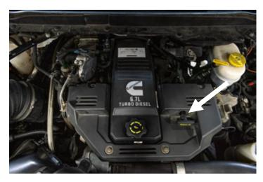
STEP 10: Remove the 4, 8 mm bolts that retain the engine shroud and remove the engine shroud.
