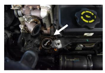
STEP 19: Install the new Fleece coolant bypass elbow into the same location as the factory coolant elbow. Install the three new M6 bolts included in the kit that retain the coolant elbow to the cylinder head. Reinstall the coolant hose and clamp.
