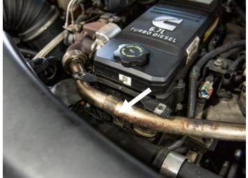
STEP 14: Remove the cross over tube and EGR cross over tube gaskets from each end of the tube. Discard the gaskets, new gaskets are provided in the kit.
