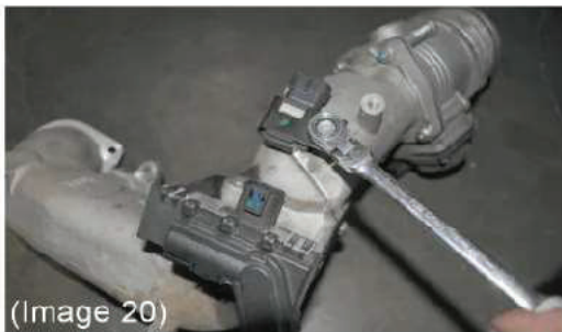
Step 29: Transfer the pressure sensor from the stock charge pipe over to the new charge pipe. The mounting bracket will need to be turned 180° on the sensor to allow mounting to the new charge pipe. (image20 and 21)
