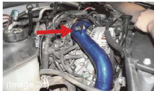
Step 29: Transfer the pressure sensor from the stock charge pipe over to the new charge pipe. The mounting bracket will need to be turned 180° on the sensor to allow mounting to the new charge pipe. (image20 and 21)
