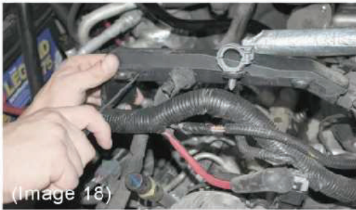
Step 27: Remove plastic cover from wiring harness to tuck harness under new charge pipe. (Image18)
