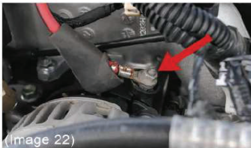
Step 30: Re-connect the charge-back wire to the top of the alternator. (Image 22)
