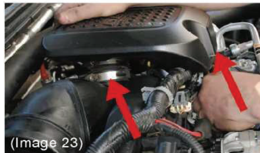
Step 31: Install the intake resonator box on top of the plastic turbo mouthpiece and secure it with the hose clamp on the bottom and the long bolt at the front of the resonator box. (Image 23)
