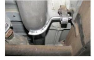
4. Starting with pipe#4121I, tighten turbo band clamp then work your way to the back connection, tightening the clamps as you go. Check for clearance.
