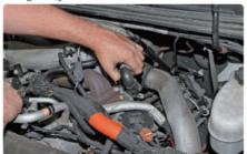
**Step 3:** To begin rerouting the factory PCV line, start by removing the crimped clamp on the line (see arrow) that connects to the valve cover below the turbo boost tube.
