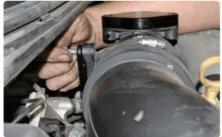
**Step 9:** Then install the included block off plate to replace the PCV hose assembly and reuse the factory mounting bolts to secure the plate. Be sure to position the wire harness bracket under the lower bolt once again so that it is secure in the engine bay as shown.
