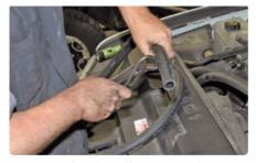
**Step 10:** Before installing the new hose on the valve cover PCV fitting, be sure to slide the spring clamp onto the hose and a few inches back from the end so that you can slip the hose onto the barbed fitting.
