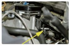
**Step 7:** But, the bottom bolt is much more difficult to access and get a wrench on. Use a U-joint socket (see arrow) and long extension along with a lot of patience to loosen and remove the lower mounting bolt.
