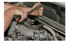
Step 2: Tightens the mounting bolts to the plate. Be sure not to over-tighten them as they are running into a plastic intake tube and the O-ring handles the seal, not the torque on the bolts.
