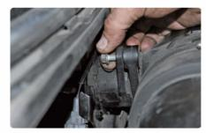
**Step 6:** After loosening the top bolt, it can be threaded out by hand.
