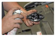
Step 1: Before installing the machined billet aluminum delete plate, lubricant on the inside and runs it around the inner edge with his finger to prevent it from snagging on the O-ring as it's installed.
