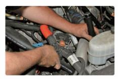
**Step 13:** With the hose secured at the fitting end, carefully route the hose to loop up and then over and down to the frame rail on the driver's side of the engine. Be careful not to route the hose near moving and/or hot items when operating the truck.
