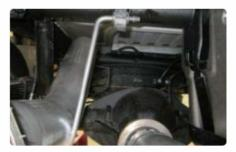
Step 4: Install tailpipe #11757 placing metal hanger into OEM isolator located in frame rail.
