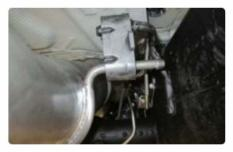
Step 3: Install muffler as well as over the axle pipe #11156, placing metal hanger into OEM isolator.
