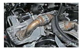
Step 19: Remove the short EGR pipe secured by four bolts. Be sure to keep all hardware and gaskets for future use. (Image 17)
