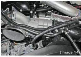
Step 16: Unplug the buttery valve located next to the fan shroud. (Image 14)
