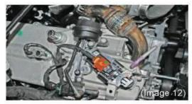
Step 14: Unplug the harness on top of the EGR cooler. The harness contains three plugs, an orange plug with a yellow locking tab, a grey plug and black plug with a metal clip. Be sure to replace the clip after unplugging it so that it is not lost. (Images 12)
