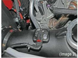
Step 3: Unplug the MAF (mass air ow) sensor that is located on the intake. Release the red tab to unlock the plug for removal. (Image 2)
