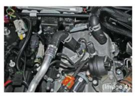
Step 8: Disconnect the clips and brackets that retain the two larger coolant lines going to the EGR Cooler. Remove the lines completely. (Images 3 and 4)
