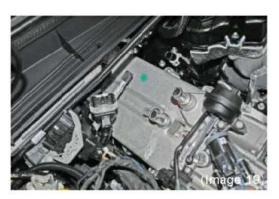
Step 21: Remove the seven bolts holding the EGR cooler in place. (Image 19)
