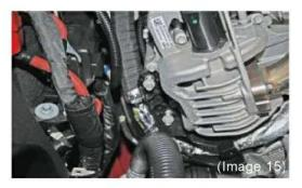
Step 17: Remove the two bolts securing the wiring harness to the EGR cooler. (Image 15)
