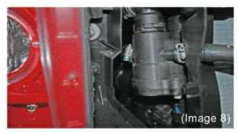
Step 10: Install the supplied coolant line from the degas tank (radiator overfow tank) to the disconnected port near the bottom passenger side of the radiator. (Image 7 and 8)
