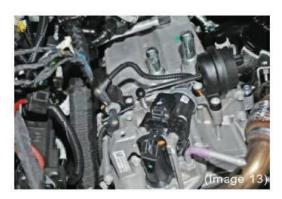
Step 15: Unplug the vacuum line on top of the EGR system pull the hard plastic line from the rubber 90 ftting cap the line with the supplied rubber cap. (Image 13)
