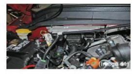
Step 13: Unplug the PCM harness from the frewall on the passenger side. Secure it out of the way for installation. (Image 11)
