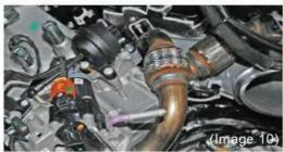
Step 12: Disconnect the EGR temperature sensor. Zip-tie the vehicle side of the plug and harness out of the way from hot or moving parts. (Image 10)
