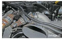
Step 9: Remove the two hose clamps on the small coolant line "T". Disconnect the lines and install the supplied straight barbed fitting. (Images 5 and 6)
