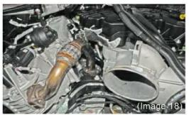
Step 20: Remove longer EGR pipe secured in place by fve bolts. Two bolts are on each fange and one is on the support bracket. Be sure to keep all hardware and gaskets for future use. (Image 18)
