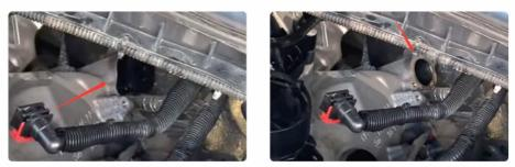
**Step 1:** Remove your current CCV outlet 2 bolt hose flange.
