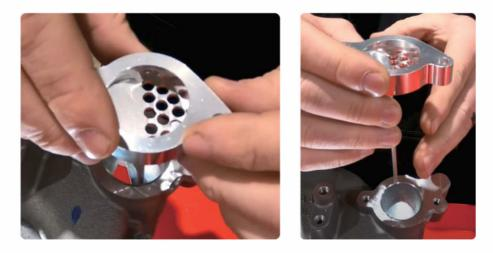
**Step 2:** Install the Internal catch can below the 2 bolt flange. Install the o ring and use the supplied longer hardware. Push the ICC towards the front of the vehicle and tighten the bolts.
