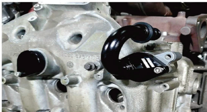
14. Correct installation as shown in the figure (slightly different from our style)
