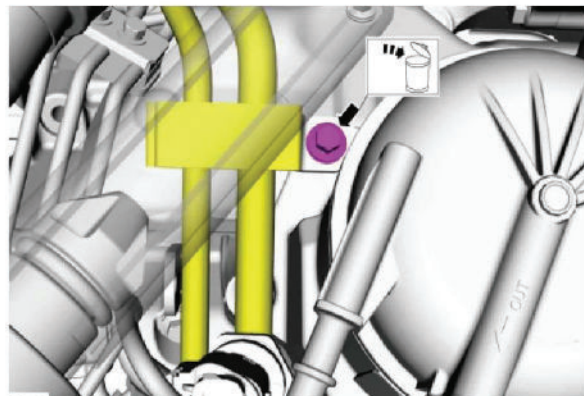
9. Remove the fuel filter and bracket assembly bolts and then remove the fuel filter and bracket assembly.
