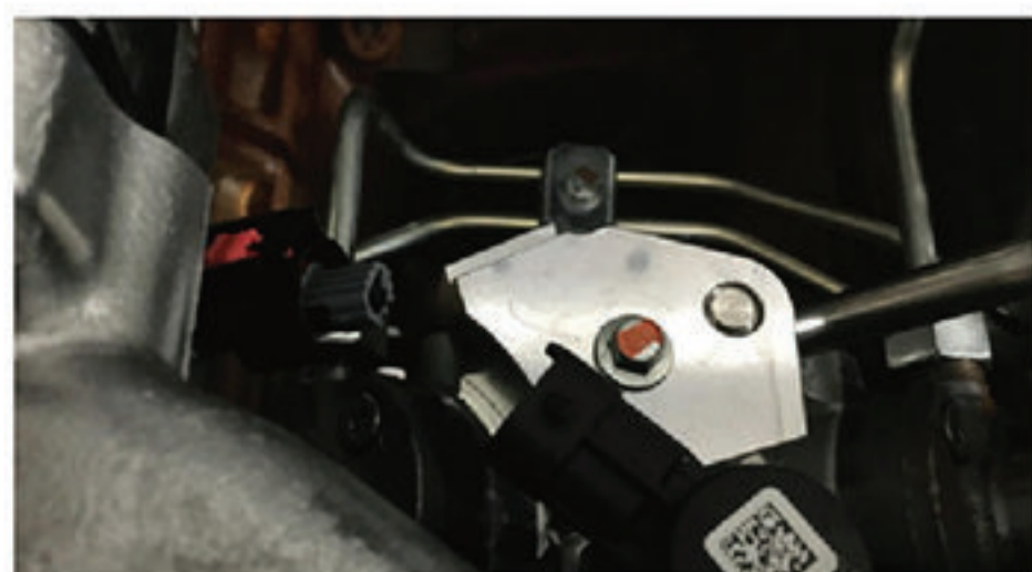
Install adapter block into pump after lubing o-rings. use caution to avoid cutting o-rings on install
