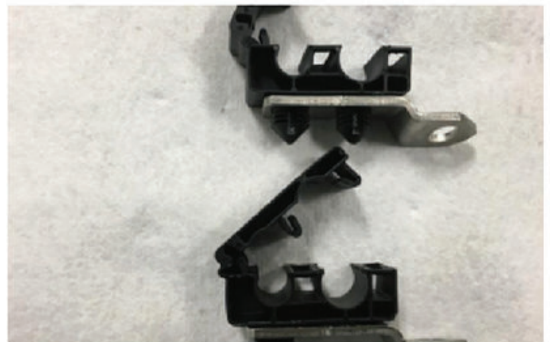
Christmas tree removed from plastic clamp to allow rotation in bracket.
