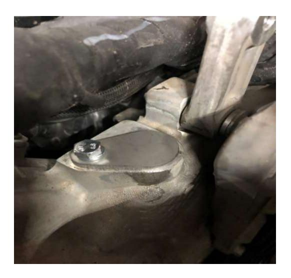
17. Now you can install the new Bypass Coolant unit. Make sure you taken the factory push in unit block off and its bare plate. Clean and dry off the block and plate add RTV and install the plate
