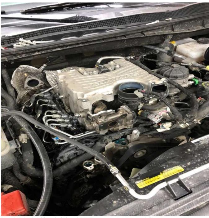
10. Now take off that back heat shield from the up pipes to give space for removal of pipes.
