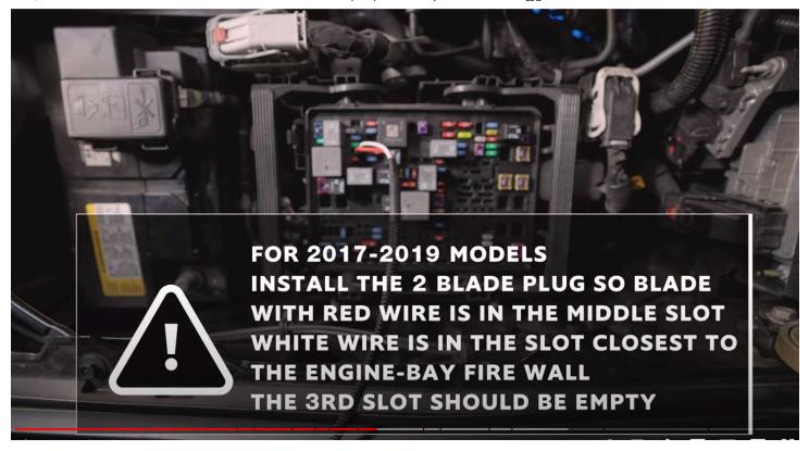
For 2020-2023 Trucks- Locate Fuse Number 78 and remove it. Install your unlock jumper into fuse spot 78 with the White Wire Facing to the drivers side. This leaves the red wire towards the engine.
