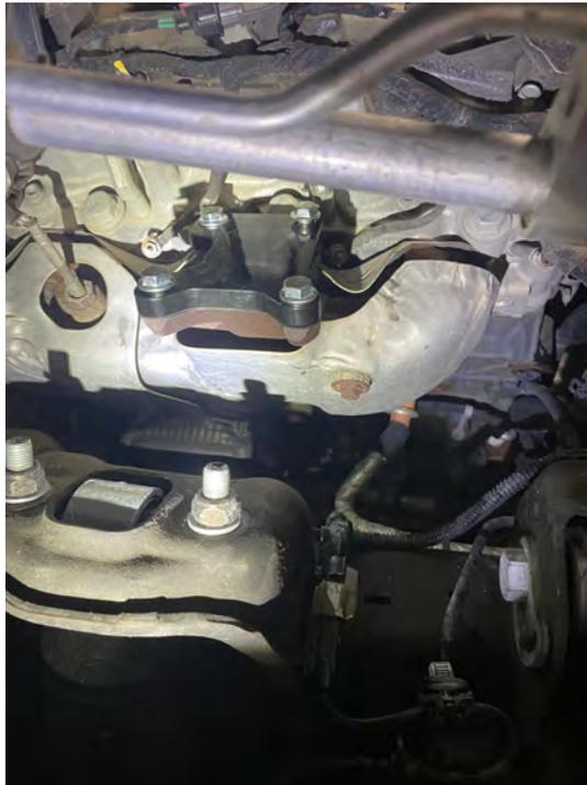
20. Next, the two large diameter steel coolant pipes from the thermostat cross over housing feeding the EGR cooler can be removed. Total of one large spring clamp just next to the turbo (leave spring clamp on this hose, it will be reused) four 10mm hex head bolts, and one 13mm hex head bolt will be removed. All circled below;
