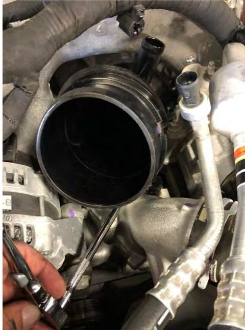
10. Remove the small diameter aluminum coolant line assembly that is bolted to the top of the Y-bridge. Leave all connecting hoses in place, just remove the aluminum hardline assembly only at this point.
