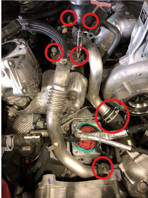
21. In the supplied parts bag of the EGR Fix Kit locate the Billet Plug with O-ring and apply grease to the O-ring, then install the plug into the coolant port on the thermostat housing just in front of the passenger side intake port. Fasten with the OEM bolt that was removed in the previous step.
