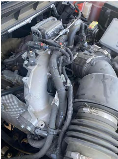
11. Next, disconnect the plastic intercooler pipe from the cast aluminum Y-bridge/throttle blade connection. This is a spring clip on the plastic cold-side pipe. Once disconnected, cover the intercooler pipe with a plastic bag or shop rag to keep anything from falling in during the rest of the project.
