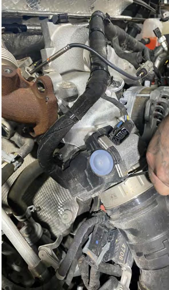
12. Now disconnect the wire harness that sits on top of the y-bridge. There are several Christmas tree style clips all along the harness and smaller connectors, remove all that are associated with the harness on top of the y-bridge so that the bridge can be removed. Disconnect the connectors on the throttle blade as well.
