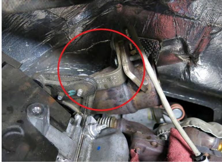
40. Remove the exhaust system front pipe and then the down pipe can be removed. It comes out easiest going down, it will require some rotation and pulling. Once out, remove the lower metal sealing ring and install this ring onto the new down pipe. If it slips off too easily from the new down pipe, the tabs on the edge of the sealing ring can be bent out slightly to help hold it in place.
