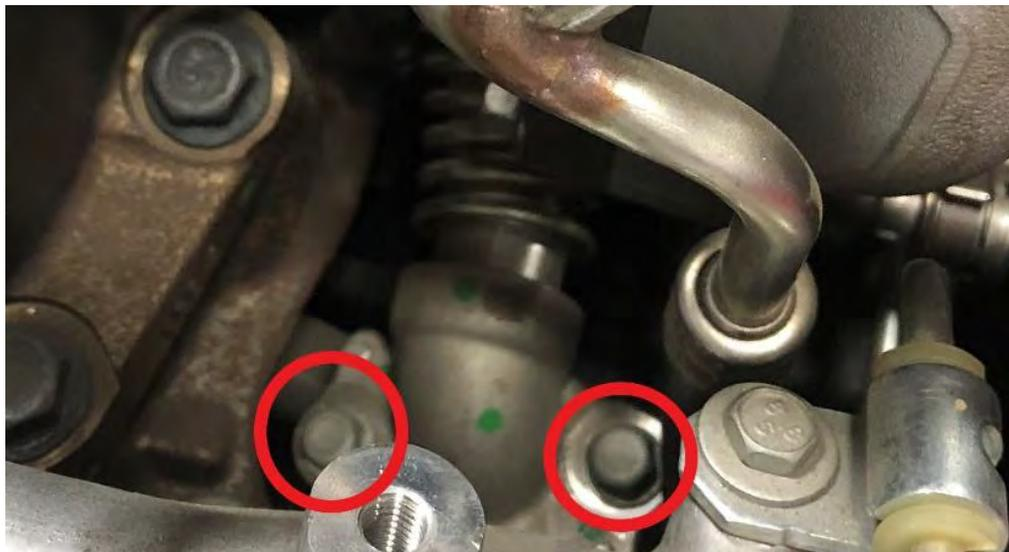
35. Now on the passenger side of the turbo, remove the four bolts that hold the coolant feed and return hardlines to the center section. These gaskets can be discarded. The feed line (lower) will stay in place, with a zip tie you can pull/tie the line forward, so it is not in the way when removing and re installing the turbo. The upper line can be set aside for install later.
