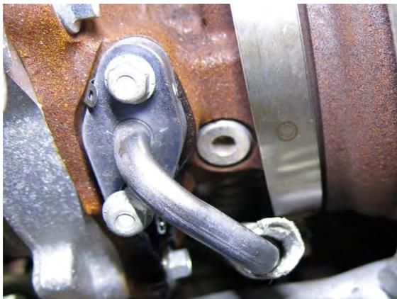
31. Remove the six bolts that hold the SCR heat shields in place, four on pass side and two on driver side. Once removed, break loose the NOX sensor on the driver side of the SCR and remove it from the SCR.
