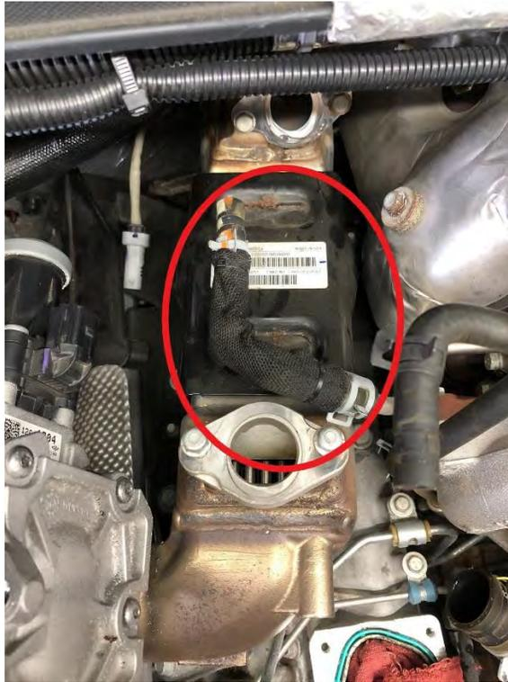
23. Then remove the five 13mm hex head bolts that hold the EGR cooler to the engine and remove the cooler assembly.
