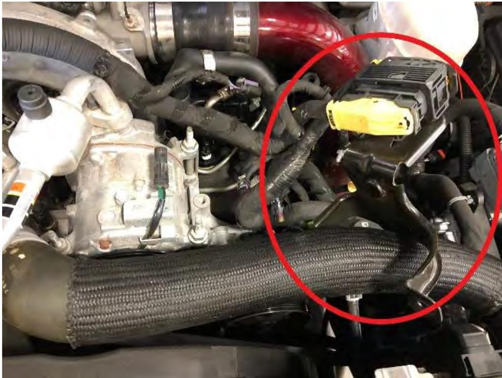
15. Remove the four 15mm head bolts holding the AC Compressor down and slide the Compressor forward towards the fan shroud so that you have better access to the Y-bridge bolts.
