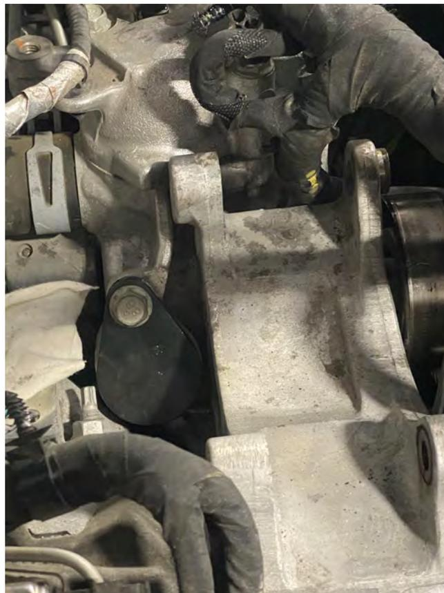
22. On the top of the EGR cooler disconnect the small coolant line from turbo to EGR;
