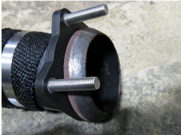
41. The new 3 1/2" down pipe can now be installed from the top side of the engine. This will also take some rotating and slight pushing but once it's in the correct spot it will drop right into place.
