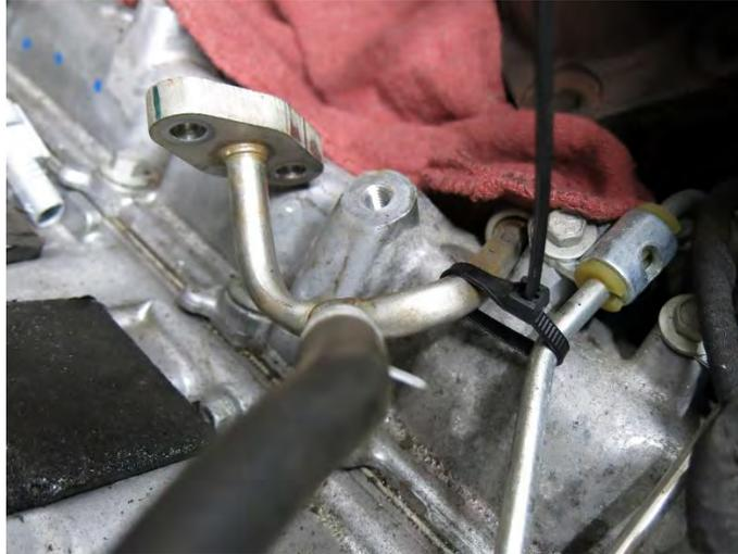
36. The four 15mm Hex head bolts that hold the turbo to the pedestal can be removed and then the turbo is ready to come off.
