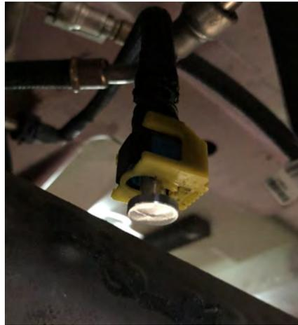
59. Reinstall the radiator coolant drain plug and refill the coolant.
