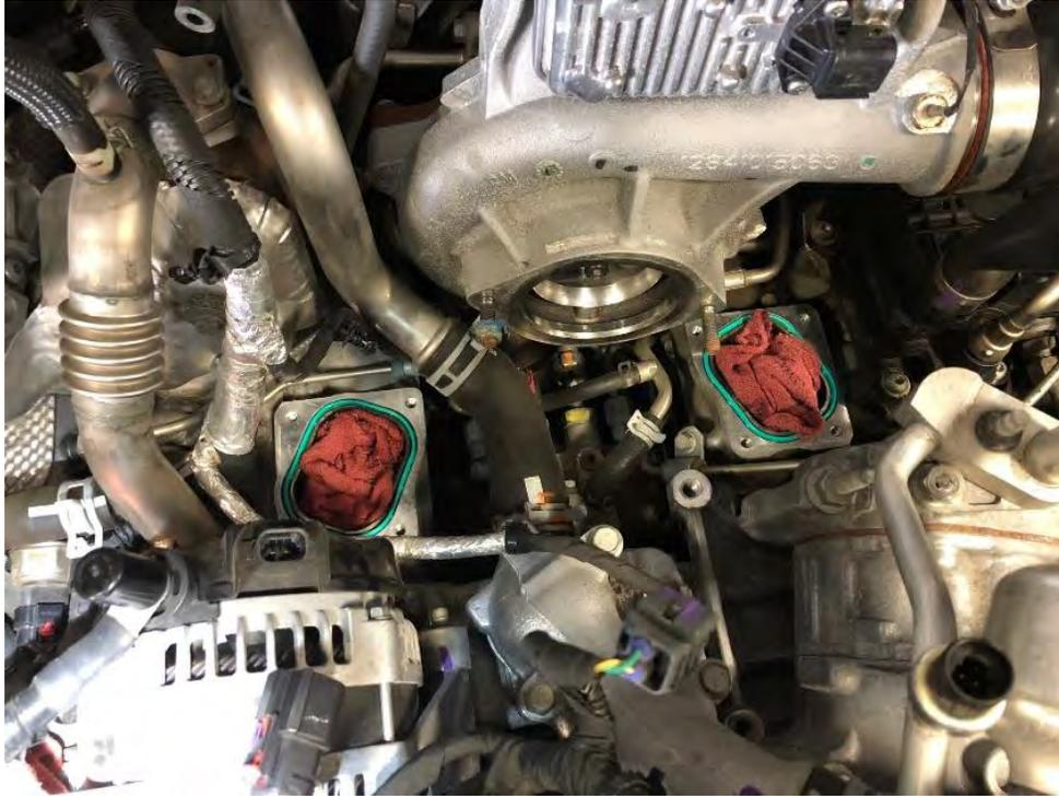
17. Now remove the heat shield on the shorter EGR hot side pipe connecting the Lower EGR valve to the Upper EGR valve, and then remove the four 13mm hex head bolts holding the pipe on and remove the pipe.
