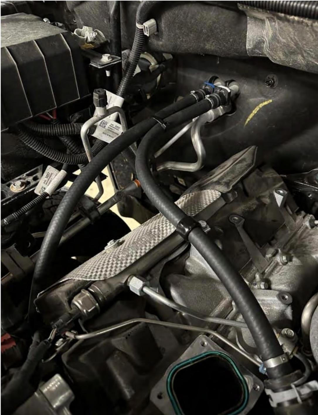
27. Disconnect the small rubber hoses at the Urea Injector located in the front elbow of the exhaust system just below the down pipe and cap the ports on the fuel cooler line with supplied HPS caps and clamps. Unplug DEF injector and tie back out of the way.
