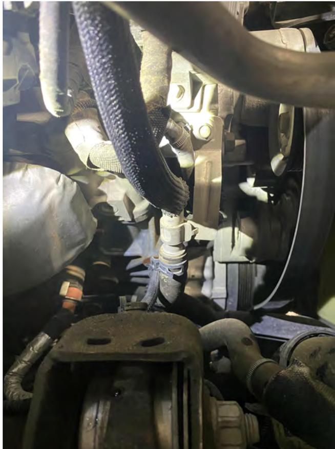
25. Now install the 32" Long, 5/8" Hose Assembly in place of the hardline that was removed above. The brass barb fitting will install to the OEM hose at the bottom with the OEM spring clamp, shown below.
