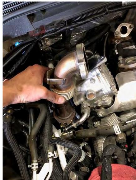
18. Disconnect all the coolant hoses at the upper EGR valve, and then you can remove the four 13mm hex bolts/nuts that hold the lower EGR valve to the exhaust manifold and then remove the lower EGR valve. NOTE: Recommend using a lube on these bolts because they are easy to break off. Tie back lower EGR valve plugs.
