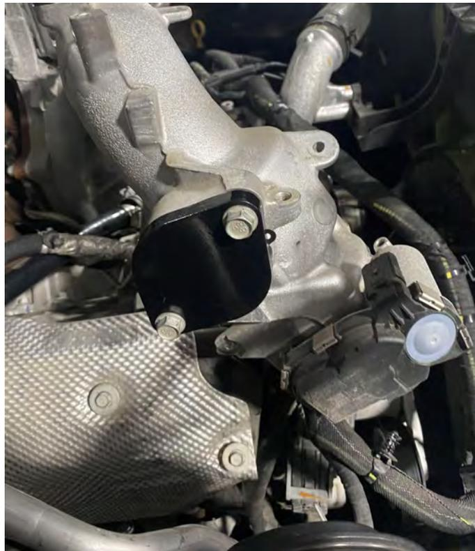
52. The intake Y-bridge can now be reinstalled onto the intake runners; be sure to remove your shop rags from the intake runner ports first! Torque the eight 10mm hex head bolts to 89 Inch lbs.
