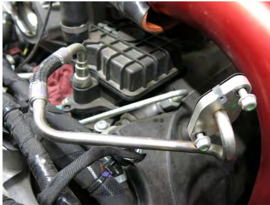
30. Next remove the two bolts on the driver side of the turbo that hold the Oil feed line to the center section. This gasket can be discarded.
