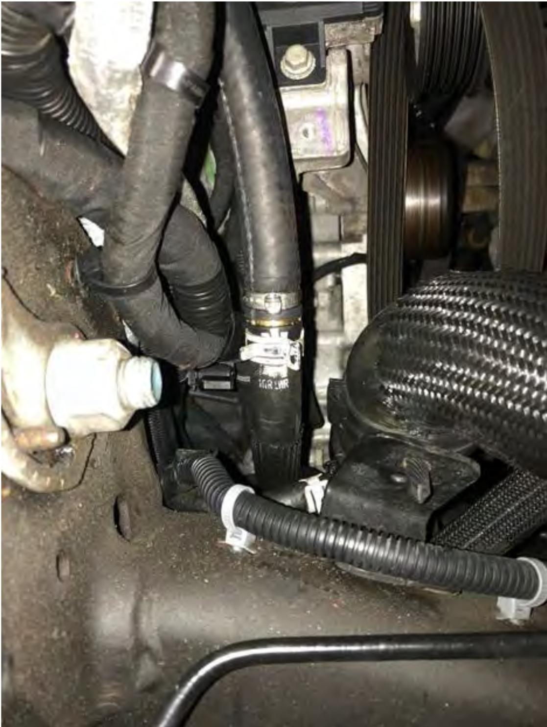
26. The upper end of the new hose assembly will quick connect to the heater core hose fitting just like the OEM hardline did, simply push together until it clips into place.
