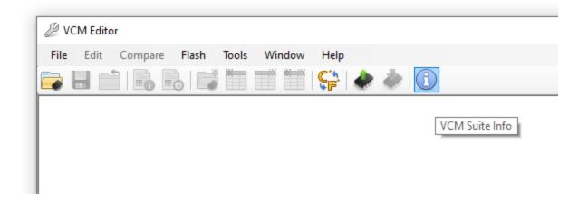
**Step 2:** Click the blue circle "i" icon to poll the software and the vehicle. Note: make sure your cable is connected to the vehicle and the vehicle's key is in the ON position before clicking the blue icon. This step may take five to twenty seconds to complete.
