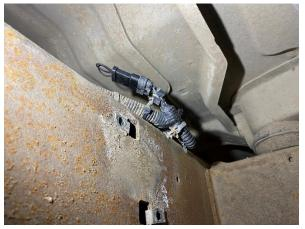
2. Install Particulate Matter Sensor Connector located on the passenger frame rail just ahead of the rear tire
